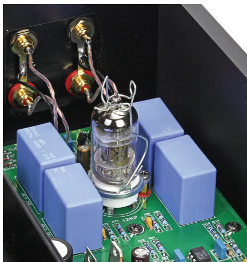
The 12AU7 is held in place by a spring clip. It is flanked by big, blue d.c. blocking capacitors.
