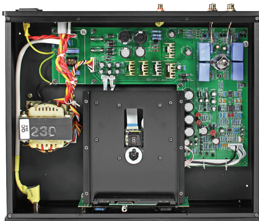
At centre lies the disc mechanism with circular hub and, above it, sliding servo-controlled carriage with laser. At top right lies the 12AU7 output Tube, as it is called in this player. The blue items are large d.c. blocking capacitors.
