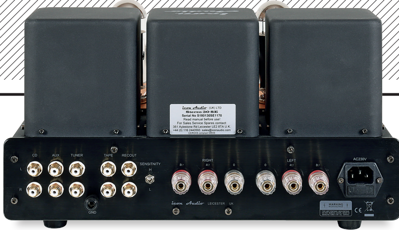
ABOVE: Two output transformers [far left/right] have dual secondaries feeding the 4 and 8ohm speaker outlets. Three line ins and a tape loop are included (no phono). The 'H'/'L' toggle offers a choice of High or Low sensitivity (or low/medium feedback)
