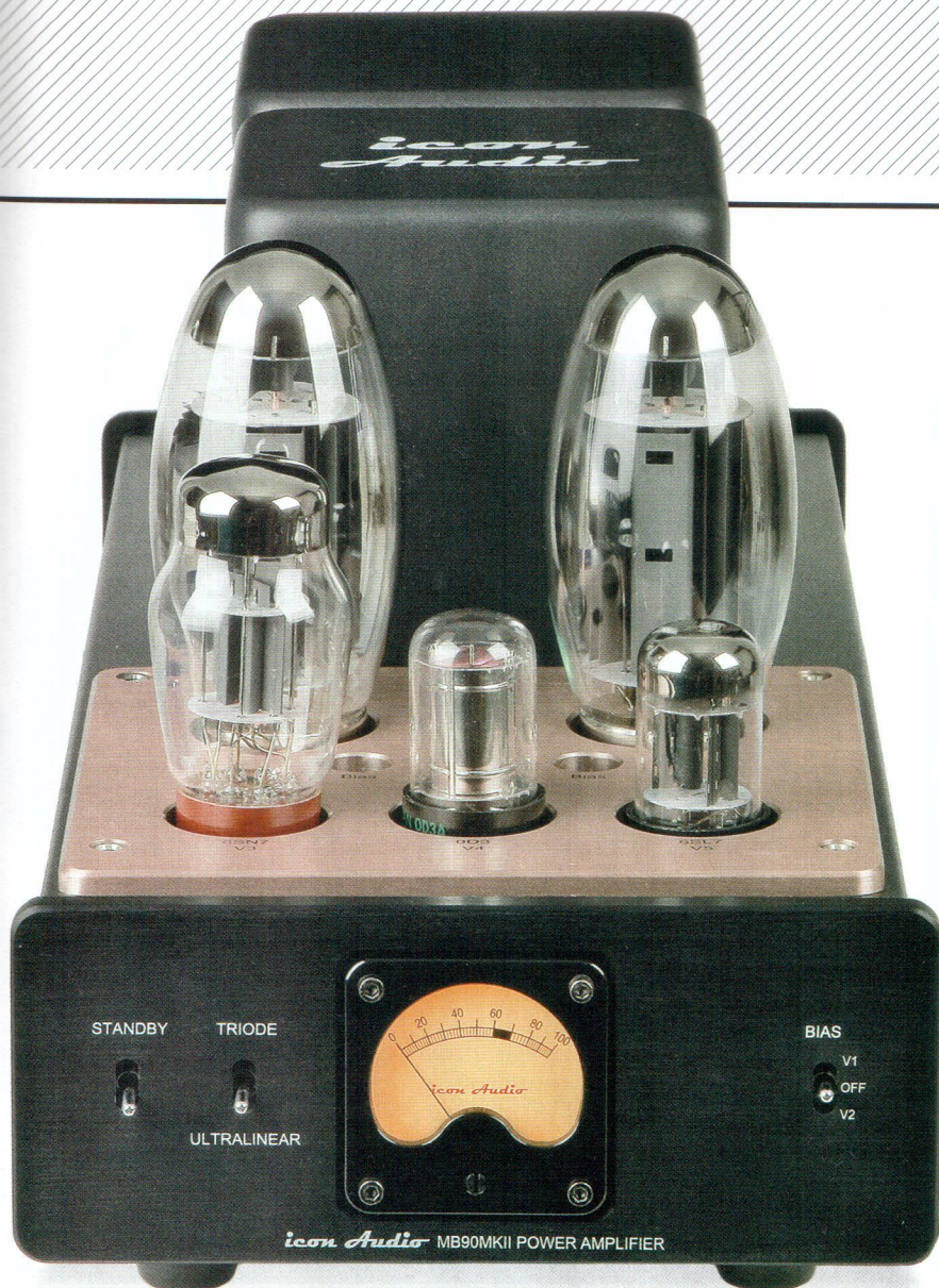
LEFT: Tung-Sol's new, egg-shaped KT150 tubes are said to give better heat dissipation, superior vacuum and freedom from microphony. They can be run in ultralinear or triode modes
