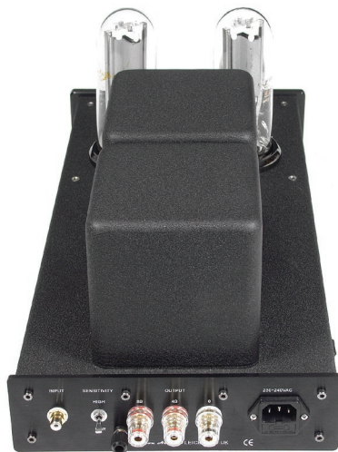
The Sensitivity switch sets feedback level. Icon Audio suggest Low Sensitivity (high feedback) is best.
